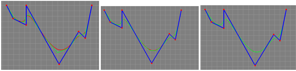
Figure 6: Subdivided curve, green in different stages. From left, subdivision 1, 2, 3. The red curve is the analytically evaluated curve for comparison.
