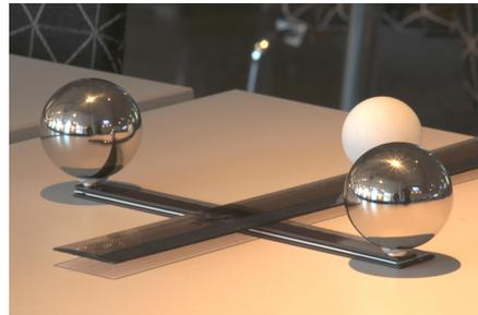
Figure 2: The setup of the dual light probes
